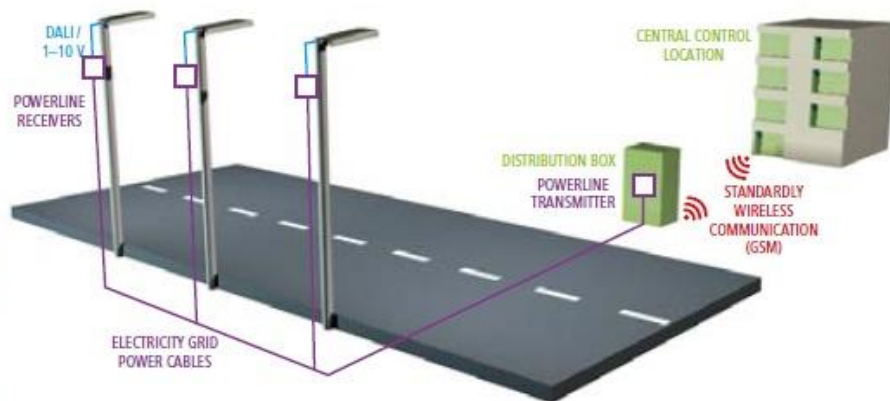
С An example of PowerLine communication.
